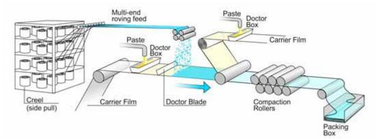
This is a mixture of resin (usually polyester), filler, catalyst and chopped reinforcing fibres (usually E glass) in 20-50mm lengths, in the form of a compounded sheet. In SMC manufacture the glass strands are sandwiched between two layers of film, which already have the resin mixture applied to them. This is then compacted and stored for several days to reach optimum properties. The sheet formed by this process is malleable but non-tacky.
