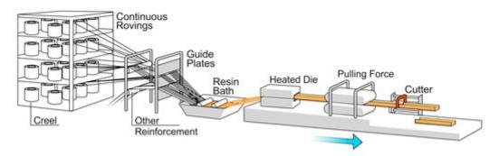
Although the mechanical properties are strongest in the machine direction (due to reinforcement fibre alignment), they can be improved in the cross wise direction by the introduction of continuous filament mat or fabrics. See also Pull Winding.
