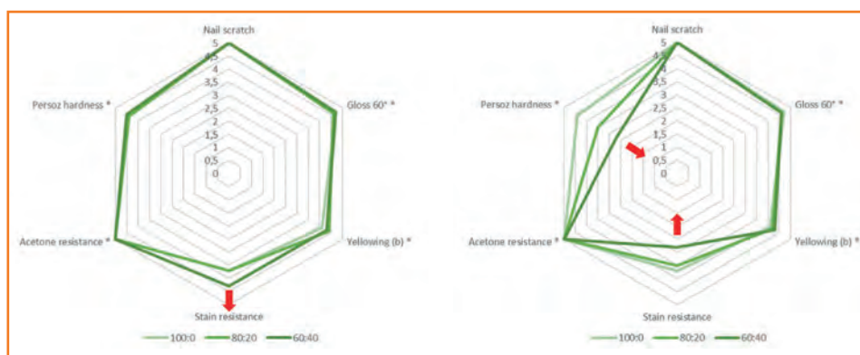
Fig. 3 (Left) Comparative normalized performance of IRR 1070 alone and formulated with UCECOAT® 7999. (Right) Comparative normalized performance of IRR 1070 alone and formulated with IRR 1074
