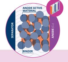
In response to market requirements for highercapacity lithium-ion batteries, allnex has developed a water-based binder that helps suppress Si-anode expansion over charge-discharge cycles.
