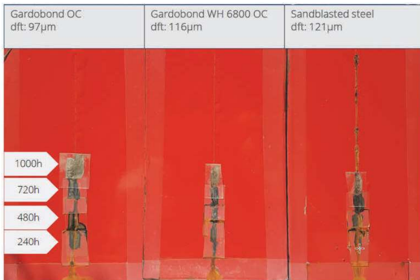
Figure 4: Salt spray testing on red pigmented topcoat based on DUROFTAL® FC 2828 for 1000 hours
