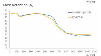
QUV B- Irradiantes = 0.75 W/m2, Condition: 50°C-4hrs UV radiation 40°C-4hrs Condensation
